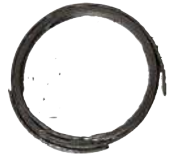
Contaminant particles from crushed graphite seal
